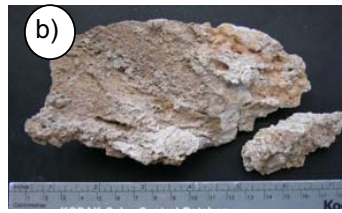
NSL TJ1 - I plaster sample: a) 1 st layer mortar b) external surface; c) internal surface
