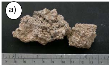
NSL TJ1 - I plaster sample: a) 1 st layer mortar b) external surface; c) internal surface
