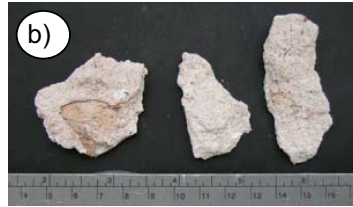
NSL TJ1 - E plaster sample: a) external surface; b) internal surface; c) polished section
