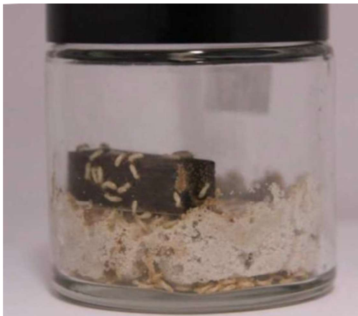
Fig. 3: Example of experimental set-up, based on a modified EN 117 test.
