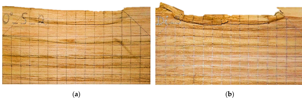
Figure 9. Crushing w perpendicular to the grain under the loaded area obtained after the tests for the sound (a) and insect-deteriorated (b) timber samples. Meshing dimensions of 5 \times 5 mm.
