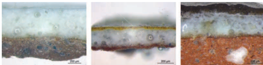
Figure 4. Polished sections of the azulejo panel Nossa Senhora da Vida observed at the optical microscope – left to right: Az032/00; Az032/03; Az032/08
