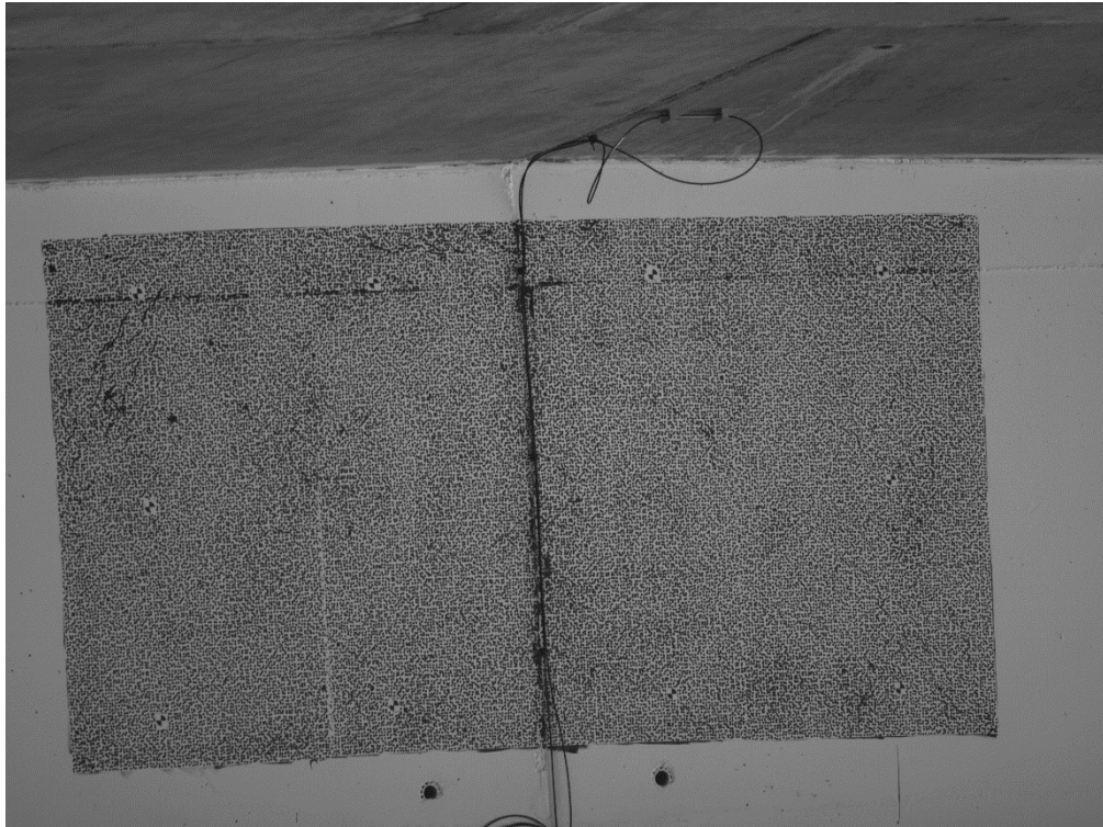
Fig. 4. Speckle pattern as seen by one of the cameras.
