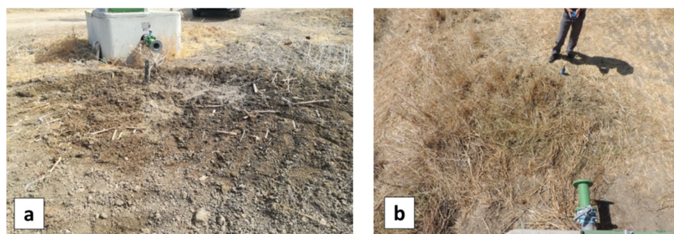
Figure 21. Artificial leaks in Ferreira district at (a) hydrant H9.7 (essentially bare soil) and (b) hydrant H16 (dry grass).
