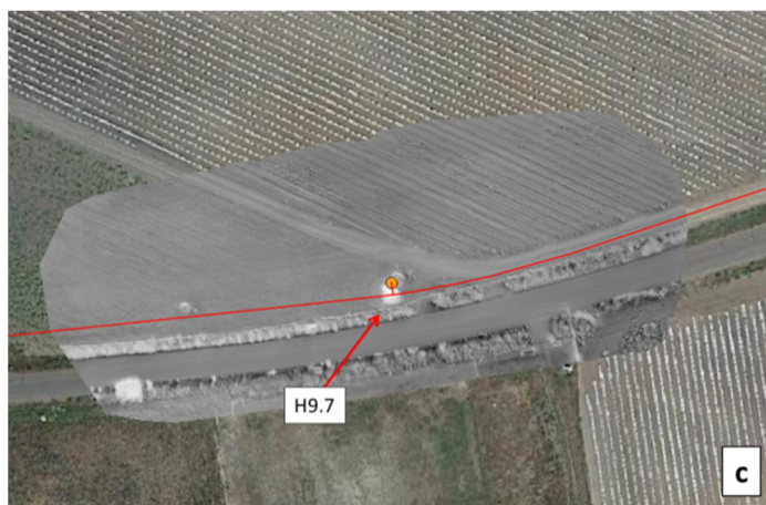
Figure 22. (a) WI image obtained with the MAV on 12 September 2019, over Ferreira district, Portugal, overlaid with the water distribution network (in red). (b) Detail of the WI image showing
