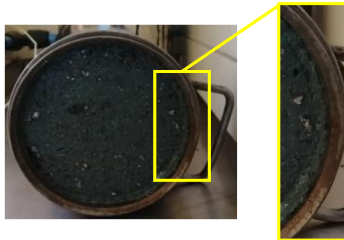
Figure 3. Blue specimen with an excess of bitumen.
