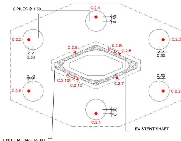
Figure 3.7: Layout of an instrumented section
