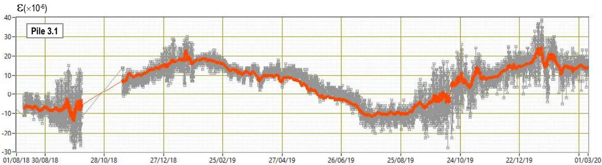
Figure 5.1: Strains in pile P3.1 of Criz II Bridge: measured values and values estimated by MLR model
