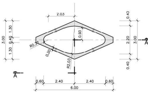
Figure 2.1: Current cross section of the piers
