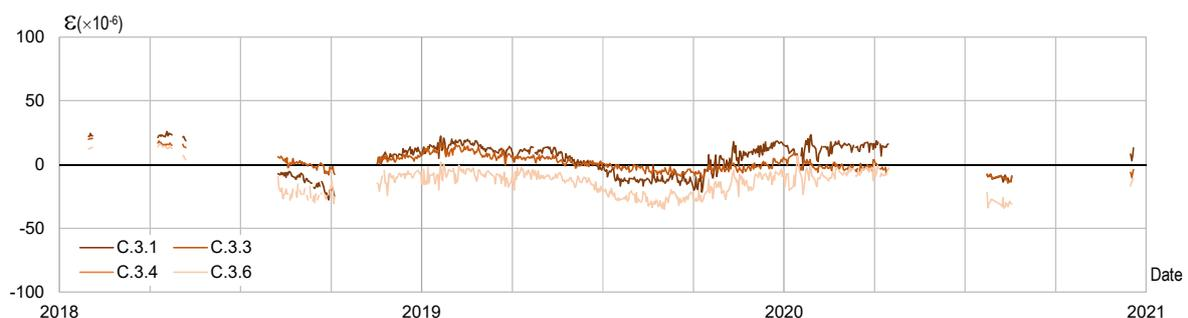
Figure 4.1: Criz II Bridge: strains measured in the piles of the pier P3
