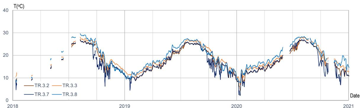
Figure 4.4: São João das Areias Bridge: temperature in the piles and in the original shaft of the pier P3
