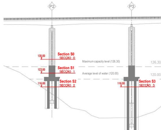
Figure 3.2: location of the instrumented sections at São João das Areias Bridge
