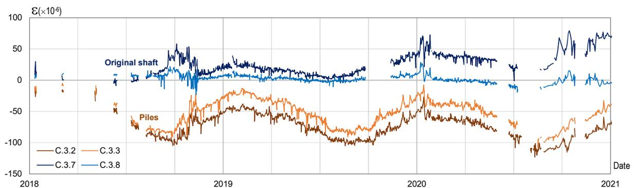
Figure 4.3: São João das Areias Bridge: strains in the piles and in the original shaft of the pier P3
