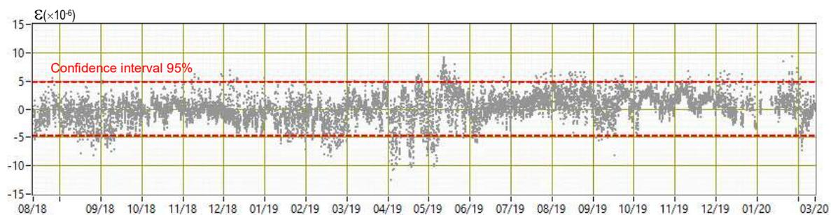
Figure 5.6: Variation of the gap at right abutment of São João das Areias Bridge: residual values of MLR
