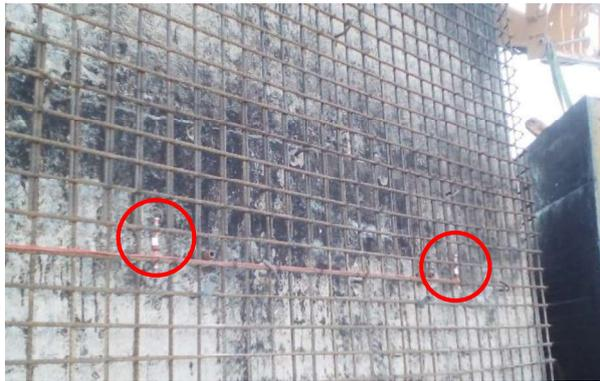
Figure 3.8: Strain gauges inside jacketing concrete
