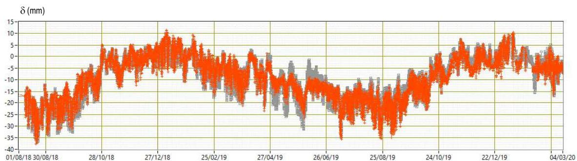
Figure 5.5: São João das Areias Bridge: measured values of the variation of the gap at the right abutment and values estimated by MLR model
