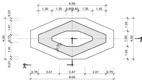
Figure 2.2: Basement and footing of the piers
