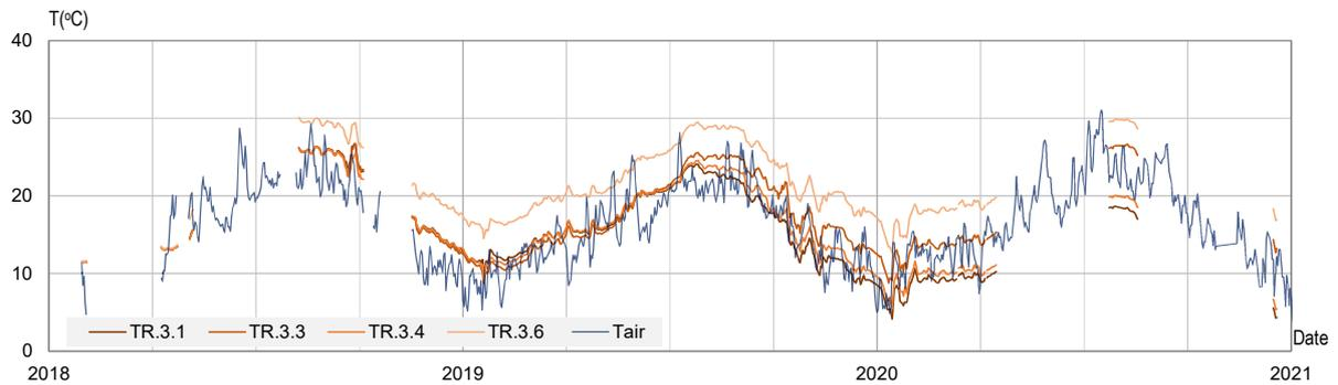
Figure 4.2: Criz II Bridge: temperatures measured in the piles of the pier P3
