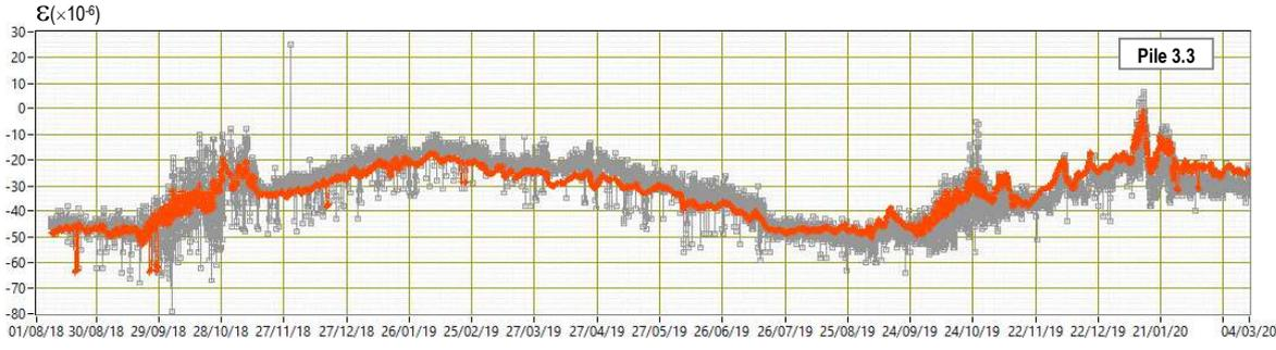
Figure 5.3: Strains in pile P3.3 of S.J.A. Bridge: measured values and values estimated by MLR model
