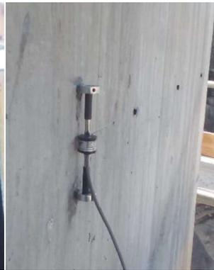
Figure 3.9: Strain gauge on the concrete surface
