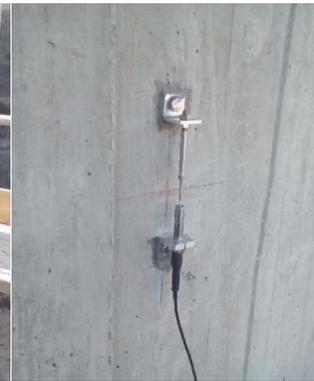
Figure 3.10: LVDT on the concrete surface
