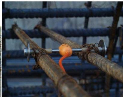
Figure 3.4: Strain gauge installed in the rebar of a pile
