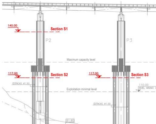
Figure 3.1: location of the instrumented sections at Criz II Bridge
