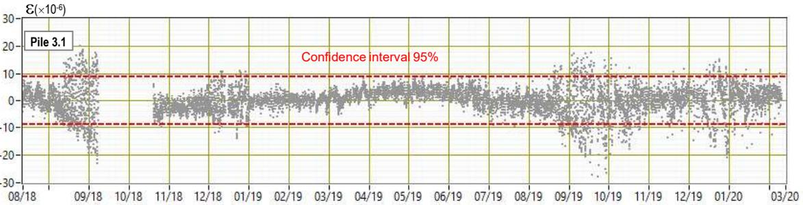
Figure 5.2: Strains in pile P3.1 of Criz II Bridge: residual values of MLR
