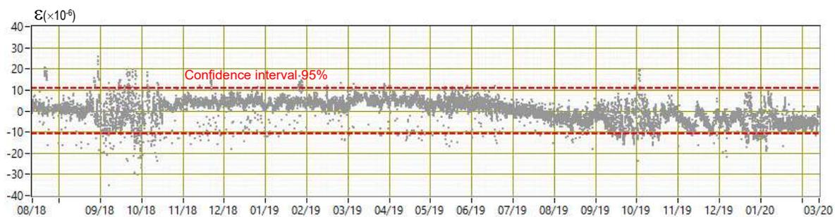
Figure 5.4: Strains in pile P3.3 of São João das Areias Bridge: residual values of MLR
