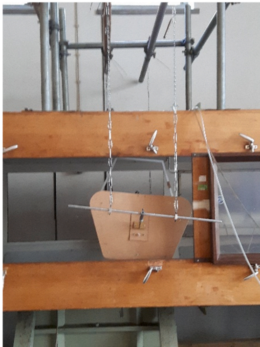
Fig. 15. Setting the angle of attacks using the suspension chains.
