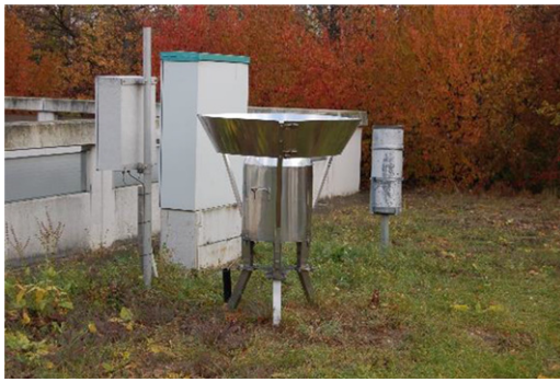
Figure 3. Weighing gauge installed in field.
