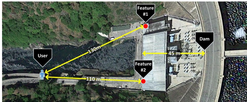
Fig. 12 - Fairly stable tracking is achievable when the user is at about 110 meters from the facade of the power plant (which is situated at around 45 meters from the downstream face of the dam), with a distance between the observer and the tracked Image Target (Feature #1), of approximately 130 meters.
