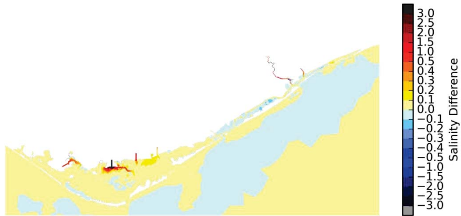
Figure 6.5 – Salinity in the Ria Formosa: differences between the sea level rise scenario and the reference scenario
