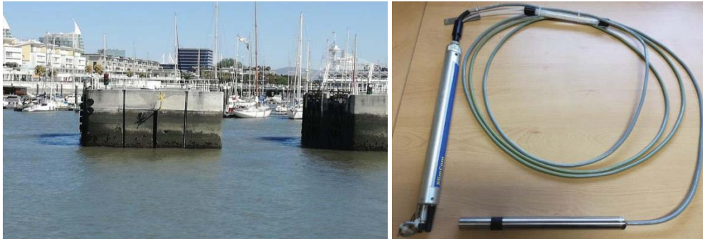
Figure 4.12 – General overview of the Parque das Nações station and SEBA MPS D3 multiparameter probe with SEBA Slimcom2 data logger
