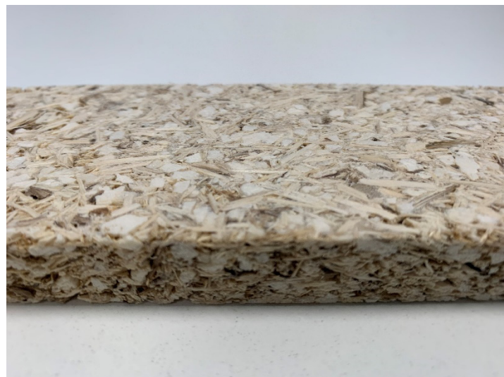
Figure 14. Cardoon particleboard with potato starch binder. Panel thickness is 16 mm.
