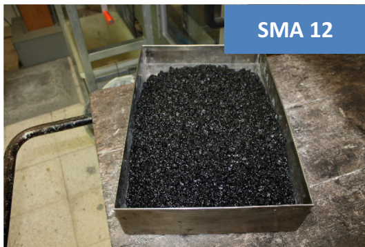
Fig. 2. Uncompact sample of asphalt mixture collected directly from the paver.
