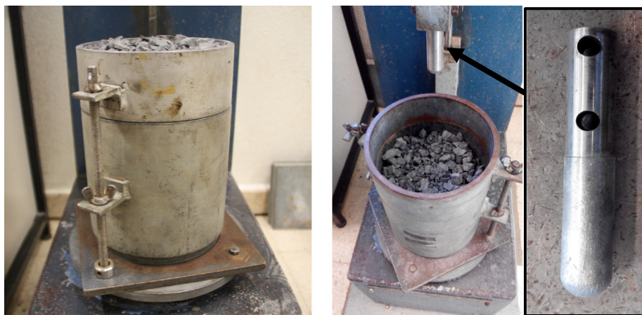
Fig. 4. Mould used and new Proctor rammer developed for tamping rod simulation.
