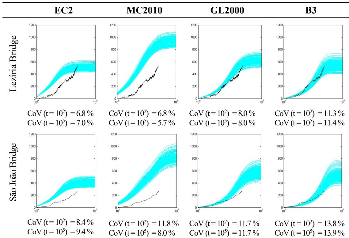
Figure 4: Shrinkage – measurements vs. model predictions.
