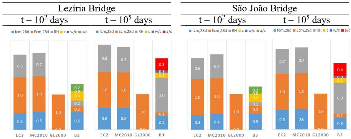
Figure 1: CoV from the sensitivity analysis on creep models.
