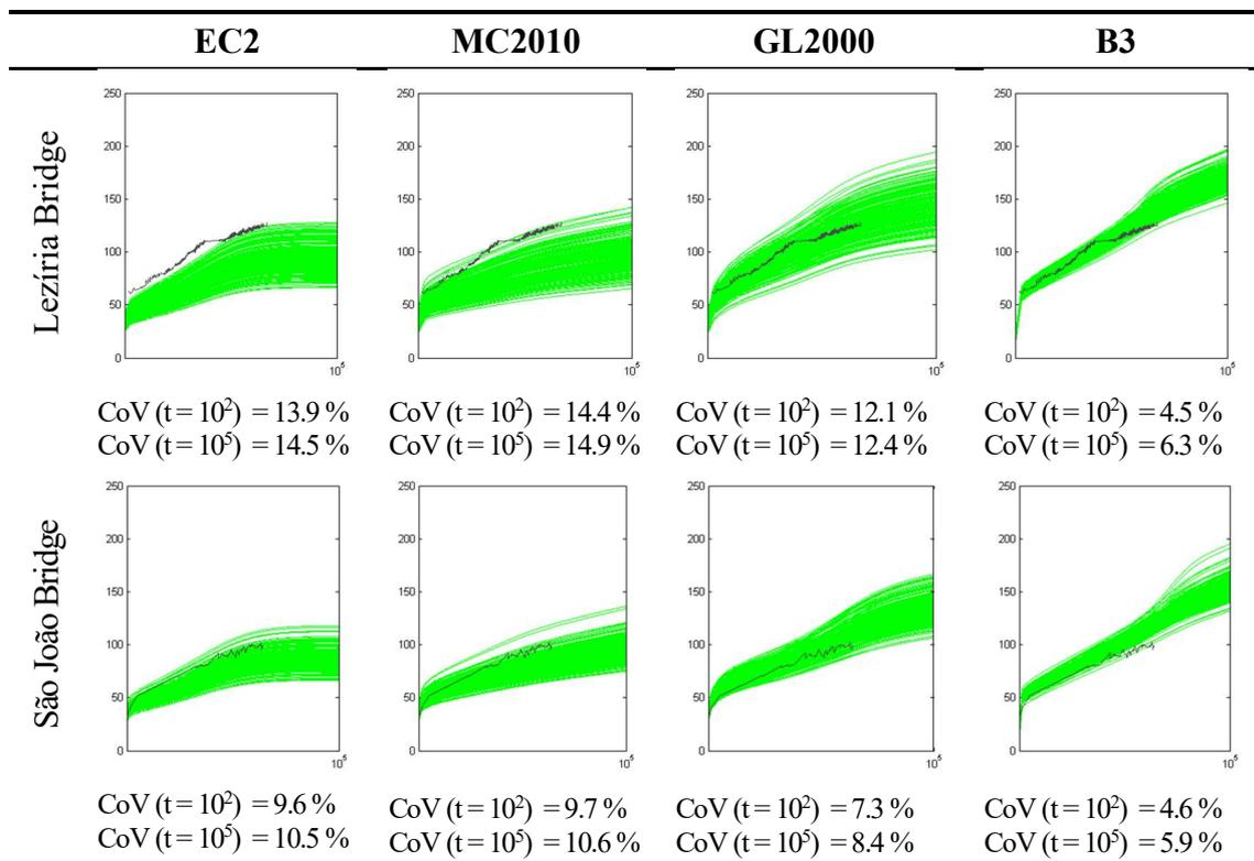
Figure 3: Creep – measurements vs. model predictions.
