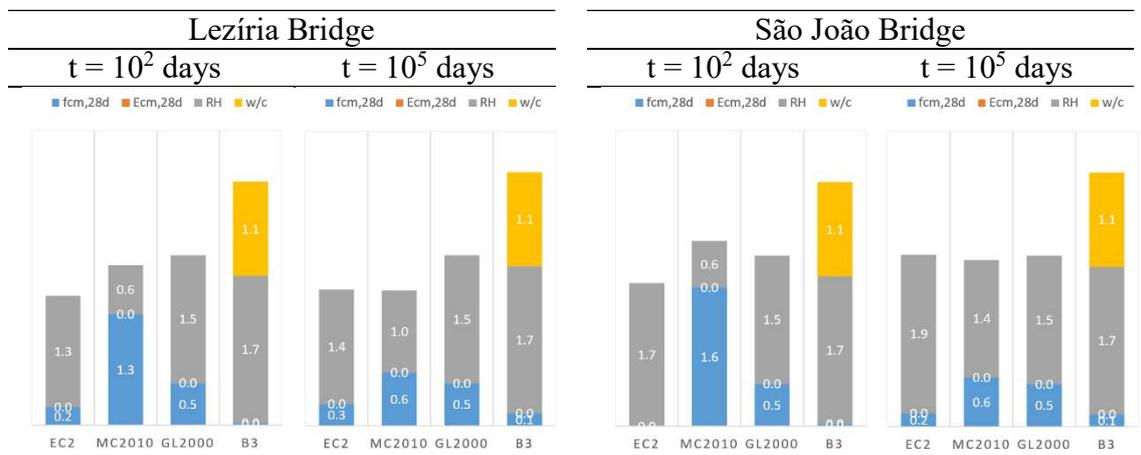
Figure 2: CoV from the sensitivity analysis on shrinkage models.
