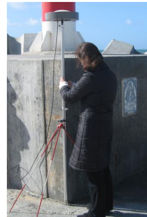
Fig.9 Coordinating a GCP using GNSS
