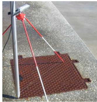
Fig. 8 Coordinating the corner of a manhole
