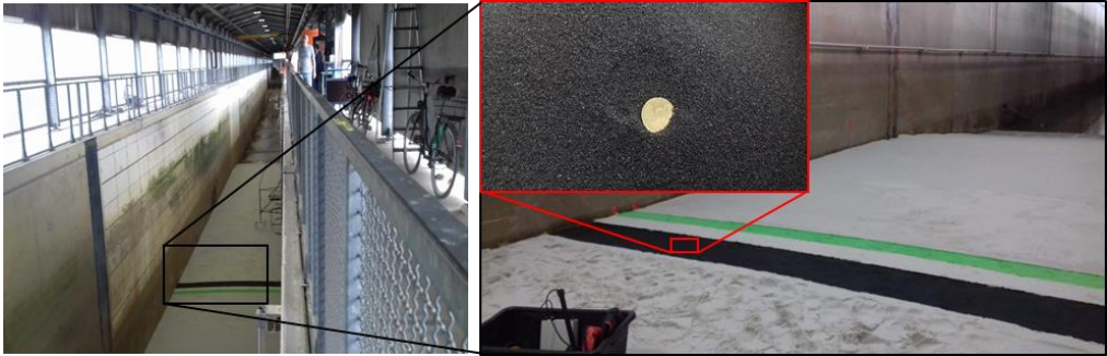
Figure 1. Test section of the experiment and the sediment tracer: green strip - fluorescent tracer; black strip - magnetic tracer.
