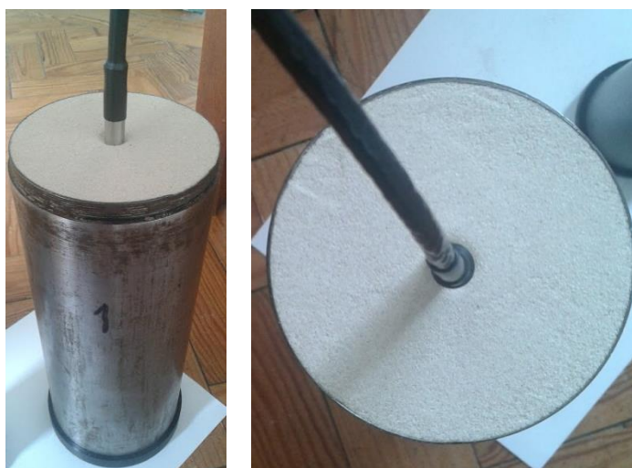
Figure 8.1 – Recipient used in thermal conductivity measurements
