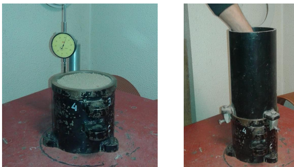
Figure 7.1 – Maximum density preparation following the standard ASTM D 4253-00
