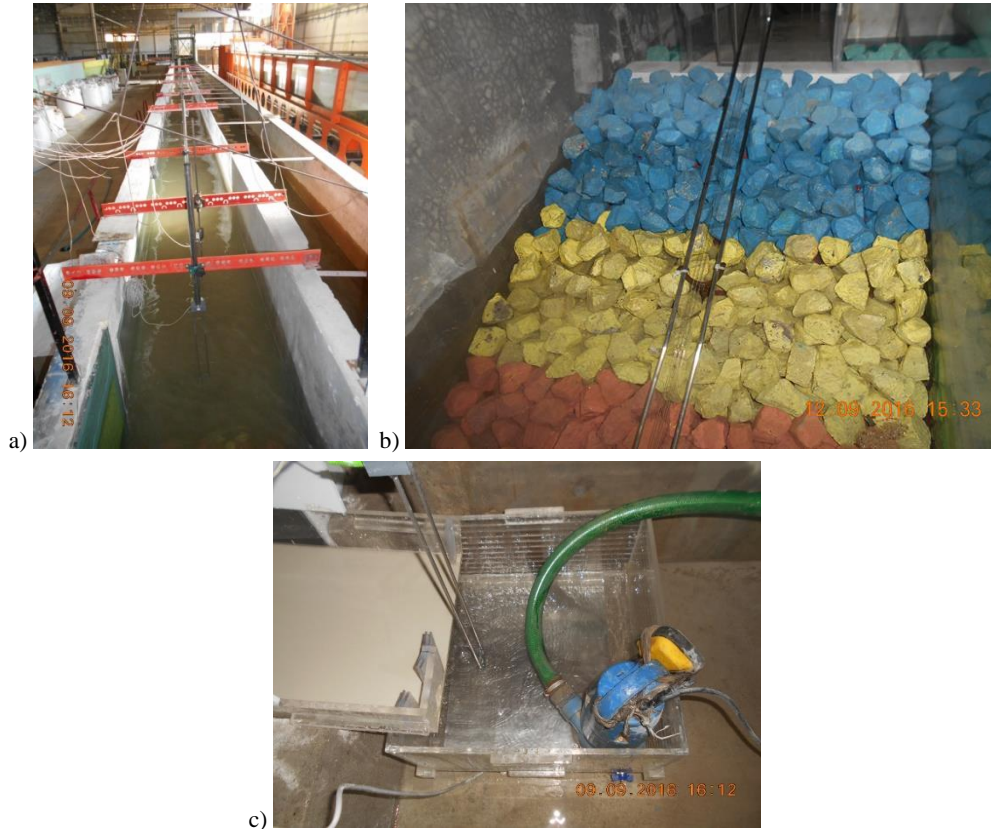
Figure 3. Measuring equipment: a) wave gauges to measure free-surface elevation; b) run-up wave gauge; c) chute, overtopping tank, load cell and water-level gauge for measuring overtopping variation.
