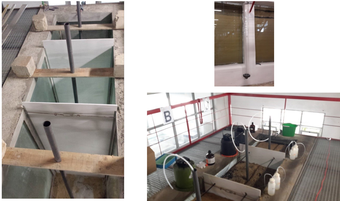
Figure 126 – LNEC physical (sandbox) model sections, A, B and C
