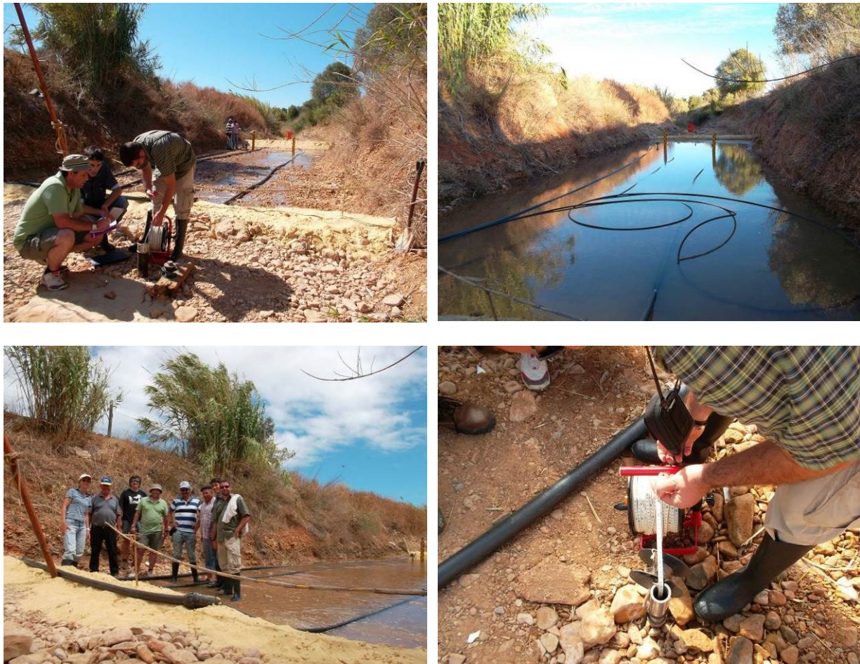
Figure 26 – Infiltration test at Rio Seco infiltration basin (PT1_1 Campina de Faro) to access clogging from 2007-2014
