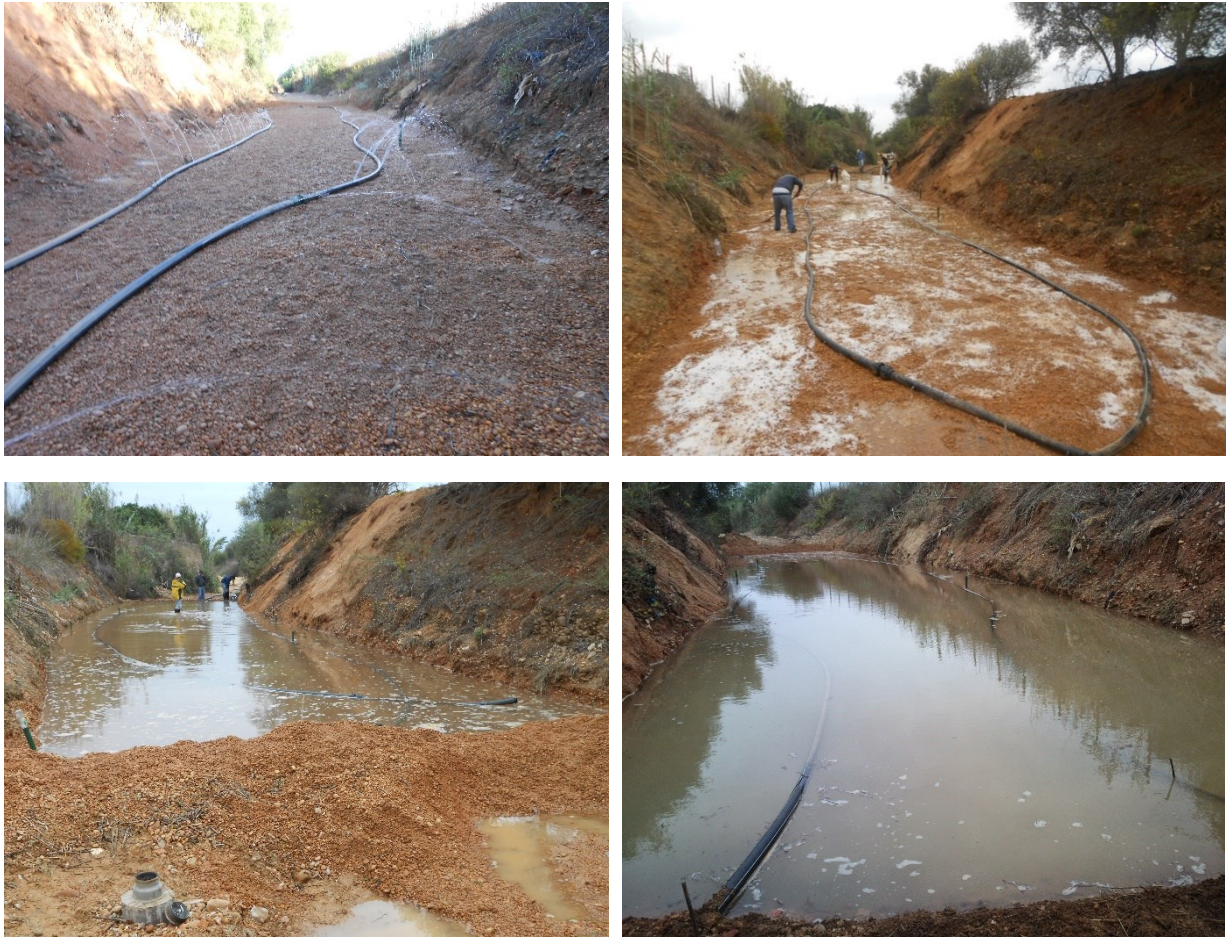
Figure 51 – Tracer test at Rio Seco MARSOL infiltration basin (PT1_2 Campina de Faro)
