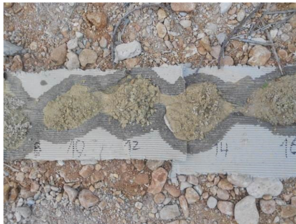
Figure 15 – Regular sample collection of materials (“cuttings”)
