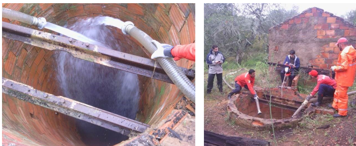
Figure 114 – Infiltration test at PT2_6 Cerro do Bardo large well with the support of Silves fire-fighters
