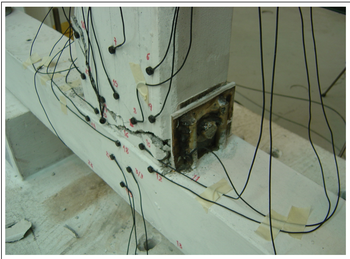
Figure C.24: Specimen V3 – Detail of the plate-beam relative displacements.
