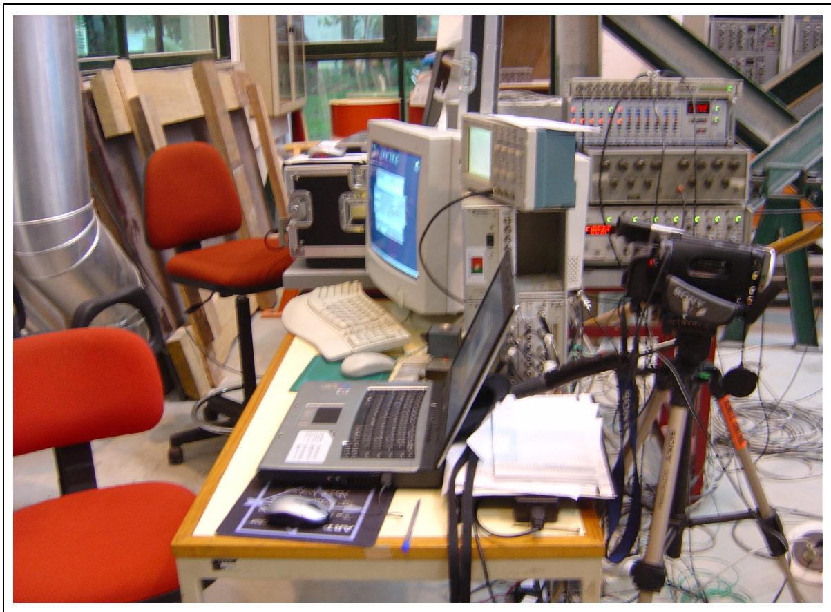
Figure C.2: Data acquisition and shaking table control.
