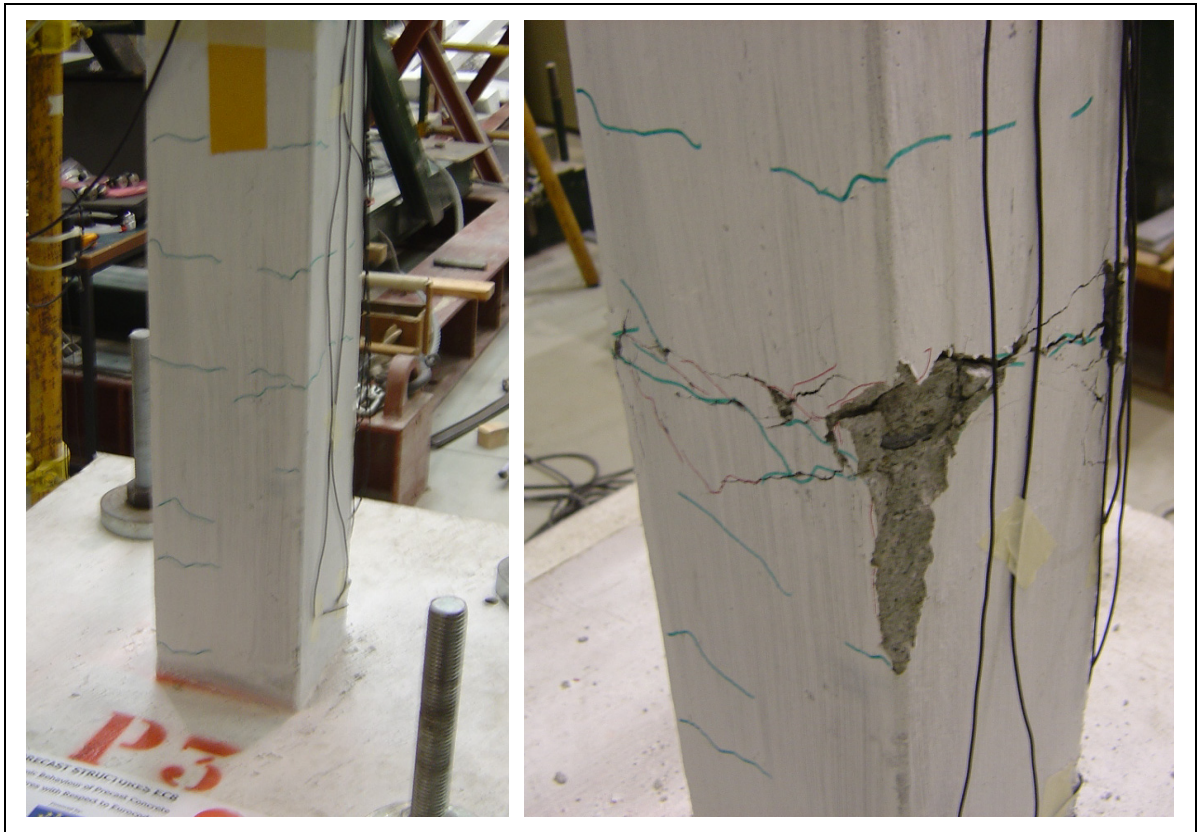
Figure C.9: Specimen P3 – Crack pattern evolution and cover spalling.
