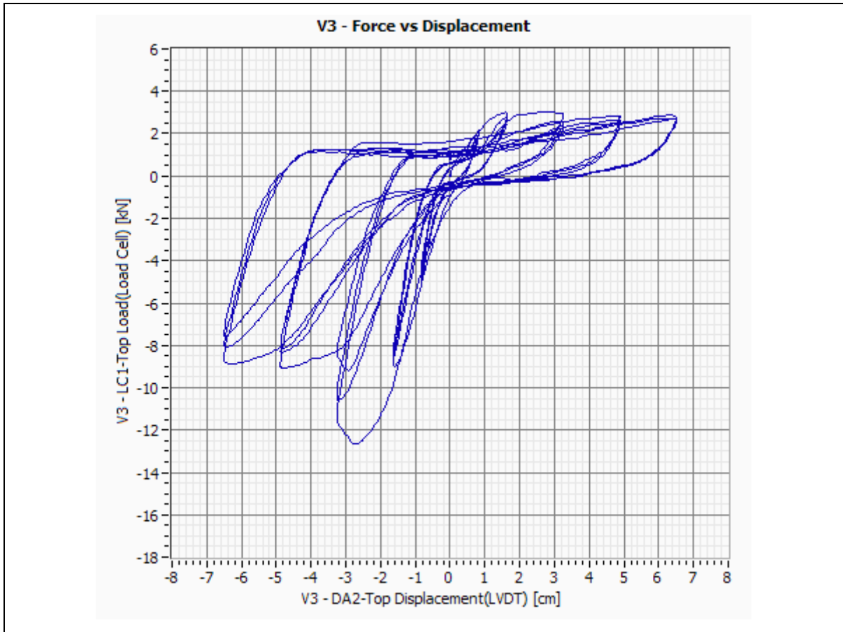
Figure E-45:– Specimen V3-Force vs. Displacement.
