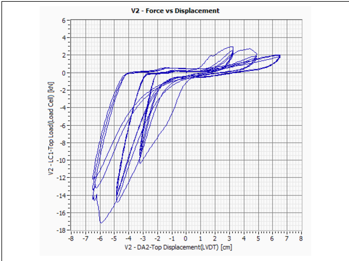
Figure E-40:– Specimen V2-Force vs. Displacement.
