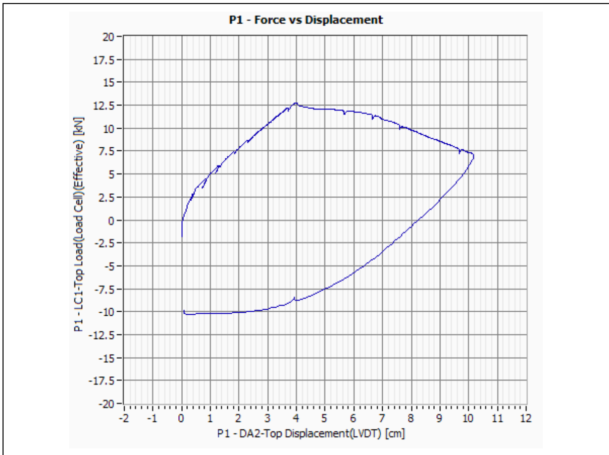
Figure E-5:– Specimen P1-Force (Effective) vs. Displacement.
