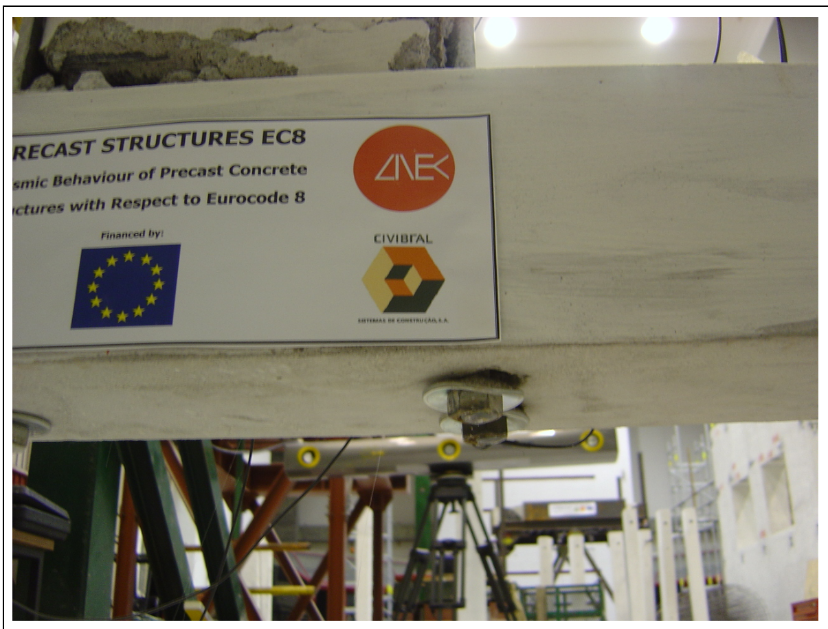
Figure C.22: Specimen V2 – Detail of the bolt's response.
