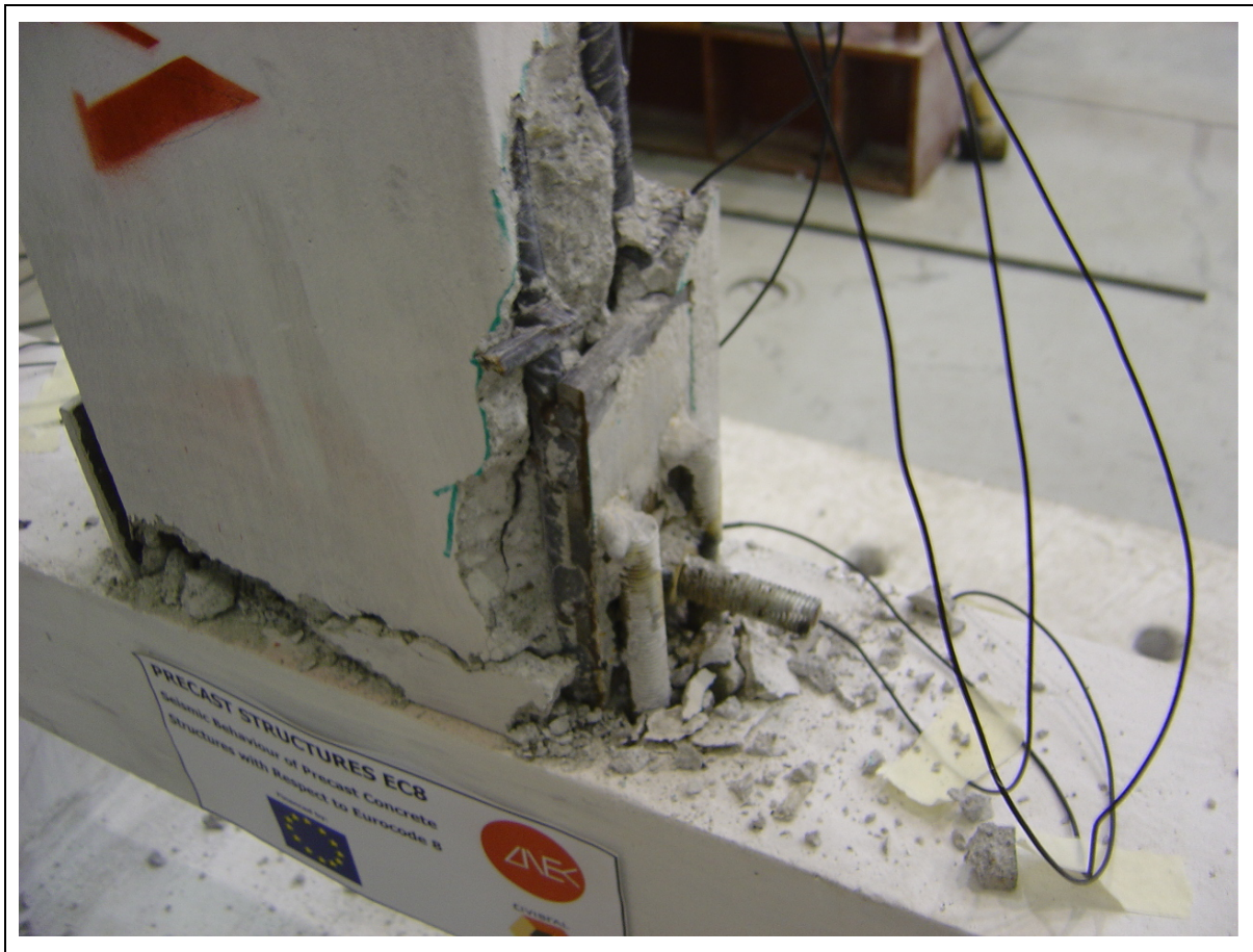
Figure C.21: Specimen V2 – Detail of the most damaged zone.
