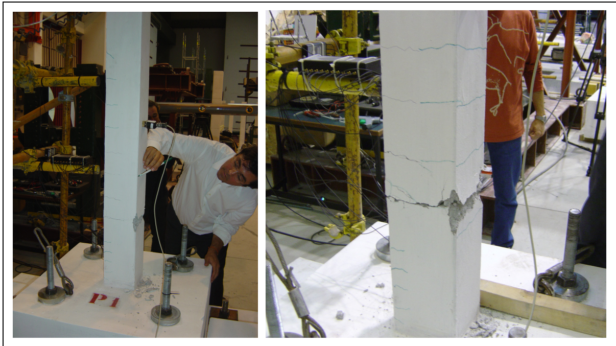
Figure C.5: Specimen P1 – Cracking evolution.
