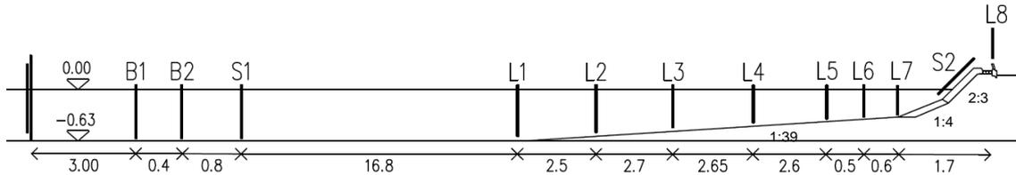
**Fig. 4 - Gauge's location along the flume - B1, B2, S1, L1 to L8 and S2 (units: m)**
