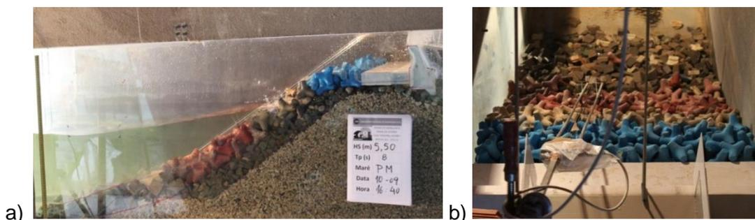
**Fig. 6 - Physical model tests: a) cross-section tested; b) run-up wave gauge**
