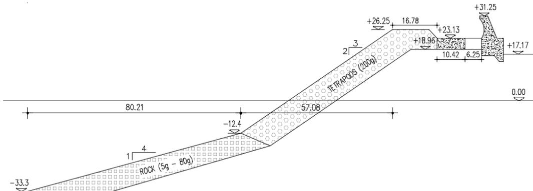
**Fig. 5 - Tested cross-section (units: cm)**
