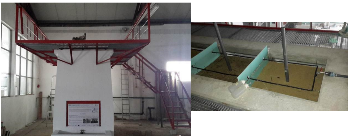
Figure 12 – PT3_7 Melides: physical sand-box (see also Task 12.5) prototype of a SAT-MAR basin, constructed at LNEC. Right: detail of the piezometers, irrigation system and vadose zone sampling cups
