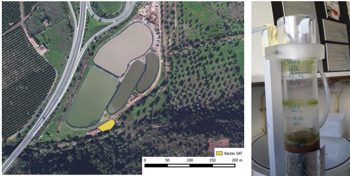
Figure 9 – PT2_4 São Bartolomeu de Messines: SAT basins location (left) and soil-column laboratory experiments set-up to access the best soil for the SAT basins (right)
