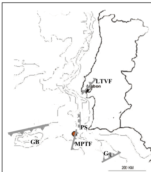
Fig. 5. Structural features. GB-Gorringe Bank (Thrust fault); MPTF-Marques Pombal Thrust Fault; Gq –Guadalquivir Bank; PS – Pereira de Sousa Fault; LTVF – Lower Tagus Valley Fault. Red circle show epicentral locations proposed by different authors and used in this study, for the Lisbon 1755 earthquake: coordinates 37°N-10°W, proposed firstly by Rodriguez [1940].
