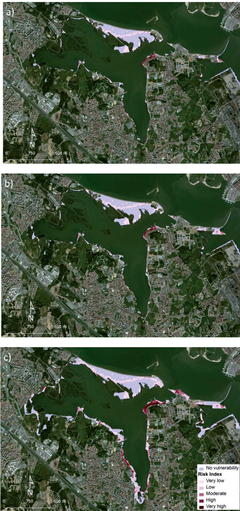
Figure 5.2 – Cartographic expression of risk index in the Seixal waterfront for different scenarios: a) 20-year return period; b) 100-year return period; c) 100-year return period with sea level rise (image: ESRI Aerial Imagery) (source: Freire et al. , 2016)
