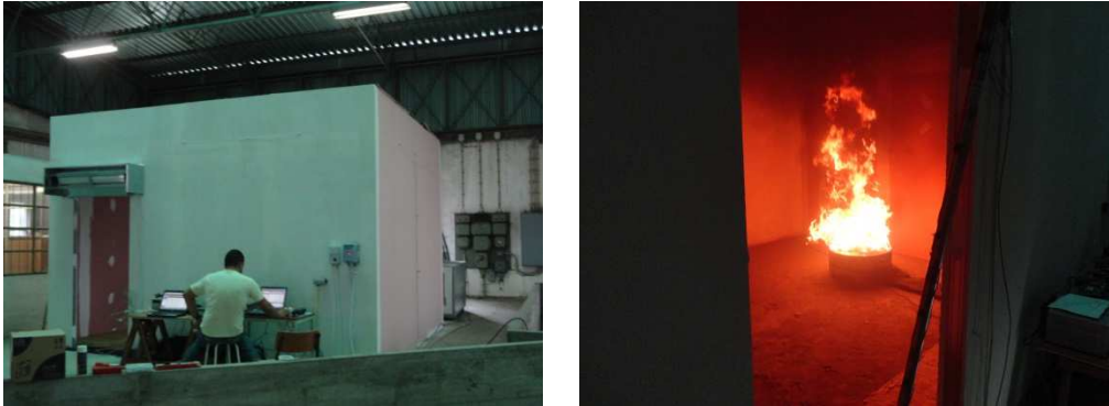
Figure 2: Perspective of the test compartment and view of the gasoline pool fire
