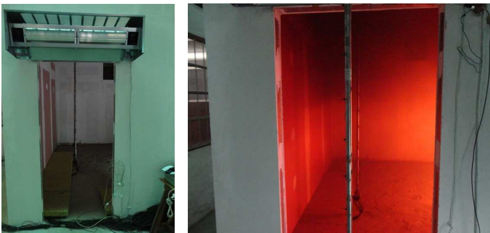
Figure 3: View of the thermocouple columns inside the compartment
