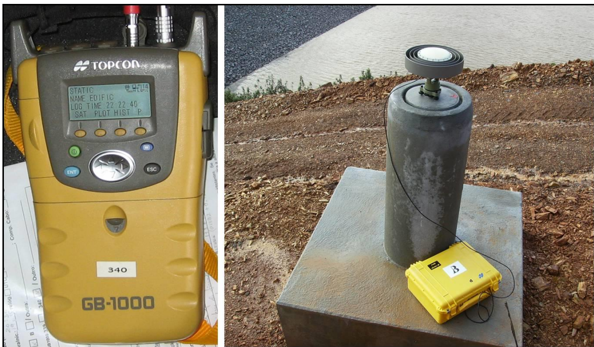
Figure 3: GNSS Receiver Topcon GB-1000 (left image) and Topcon GNSS Choke Ring antenna TPSCR3_GGD stationed in one of the reference pillars of surveying observation system of Odelouca Dam (right image).
