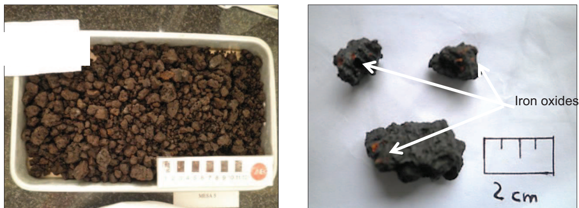
Figure 7. ISAC/gravel after permeability test with leachate
