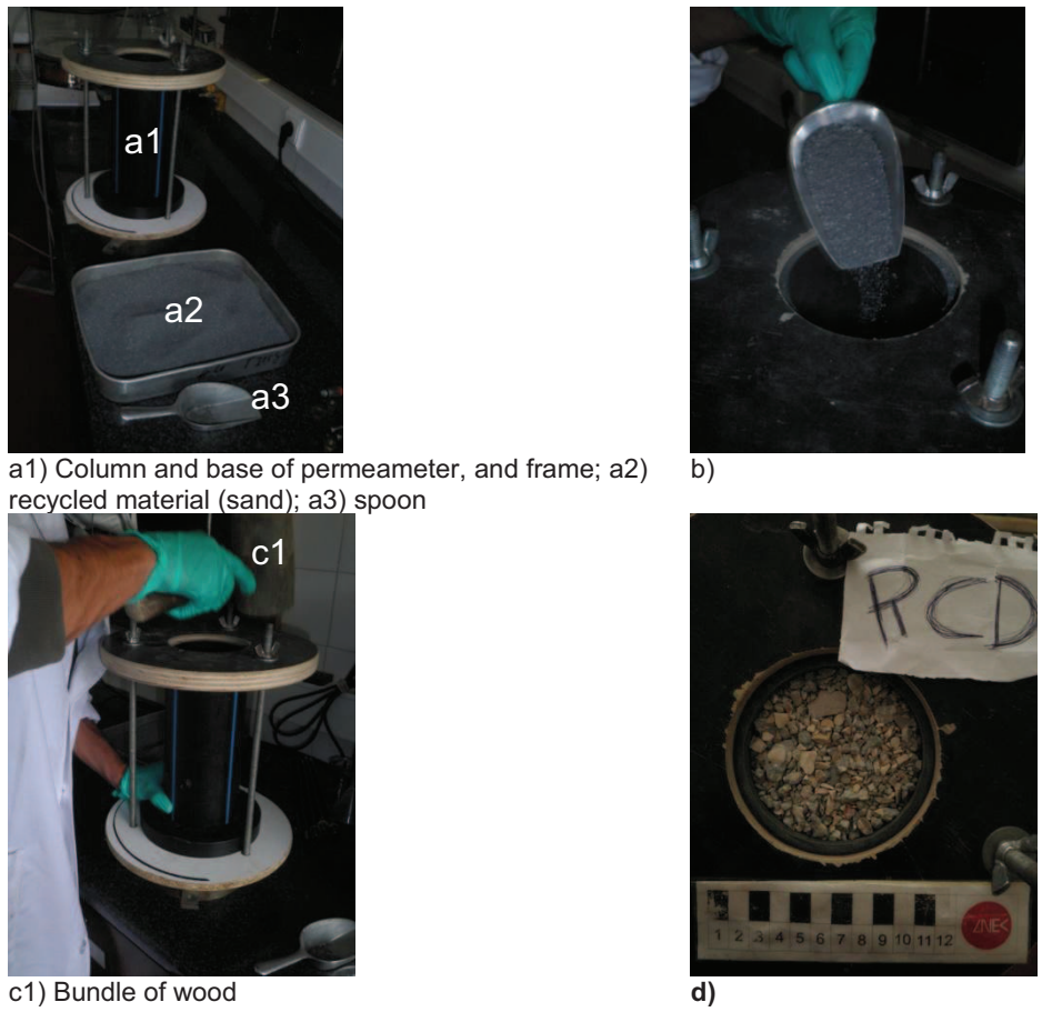
Figure 4. Procedure adopted for filling the columns of permeameters
