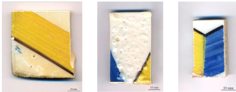
Figure 6. Visual observation of double-stage re-firing results: a) not re-fired; b) single-stage refiring (990°C 5 minutes); c) double-stage re-firing
