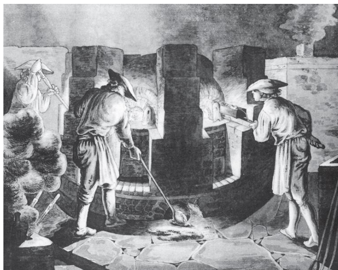
Figure 6- The hard work under the heat of the glass furnace. The melting of smalt was made in pots of clay at 1100 to 1250 ° C. The worker at right feeds the oven while at left the molten smalt is taken.
