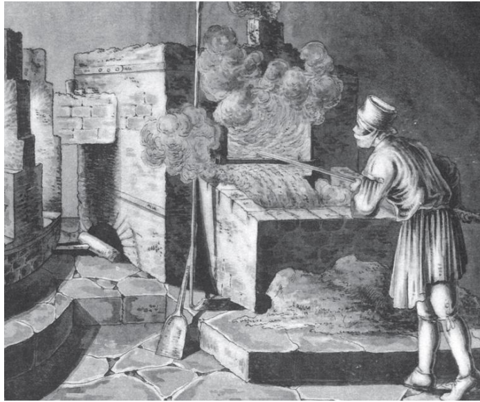
Figure 5- Roasting of the cobalt ore. Most of the unhealthy sulfur and arsenic fumes were channeled and condensed inside constructions called “smoke chambers” however the workers still had to cope with part of them.
