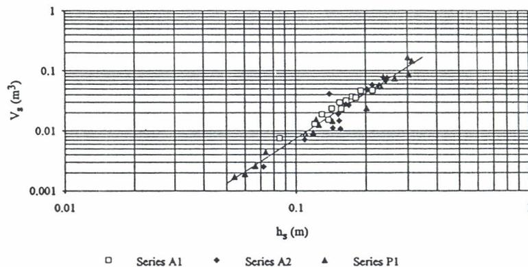
Fig. 3 - Excavated volume due to local scour
