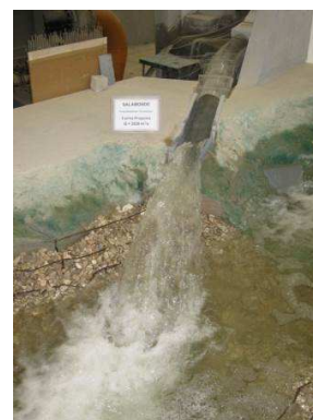
Figure 13: Ski jump structure with proposed shapes. Design discharge ( 2828 \text{ m}^3/\text{s} )
