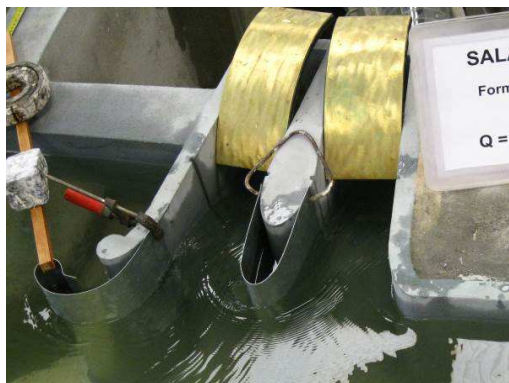
Figure 10: Control structure with one of the alternative shapes. Design discharge ( 2828 \text{ m}^3/\text{s} )
