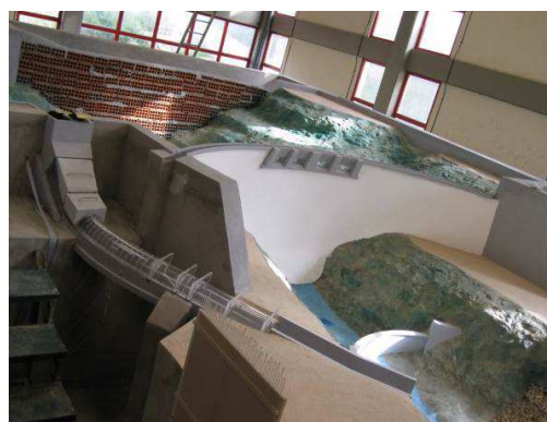
Figure 7: Hydraulic model. Downstream view
