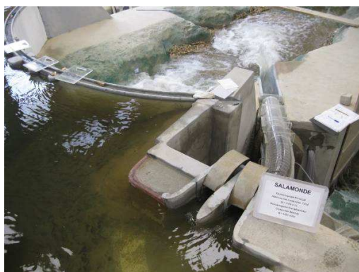
Figure 12: Control structure with proposed shapes. Design discharge ( 2828 \text{ m}^3/\text{s} )
