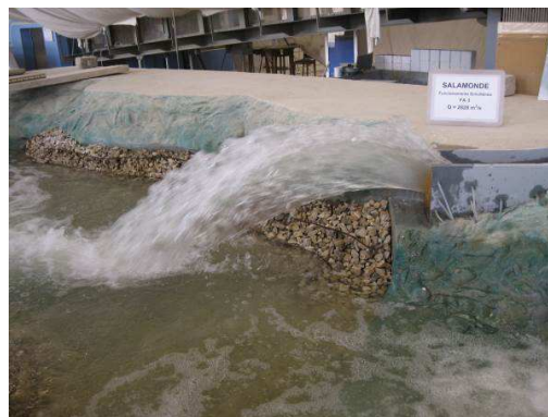
Figure 11: Ski jump structure with one of the alternative shapes. Design discharge ( 2828 \text{ m}^3/\text{s} )
