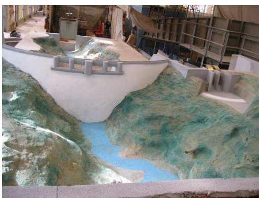
Figure 6: Hydraulic model. Upstream view
