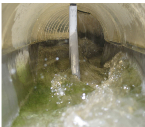
Figure 14: Physical model flow inside the tunnel
