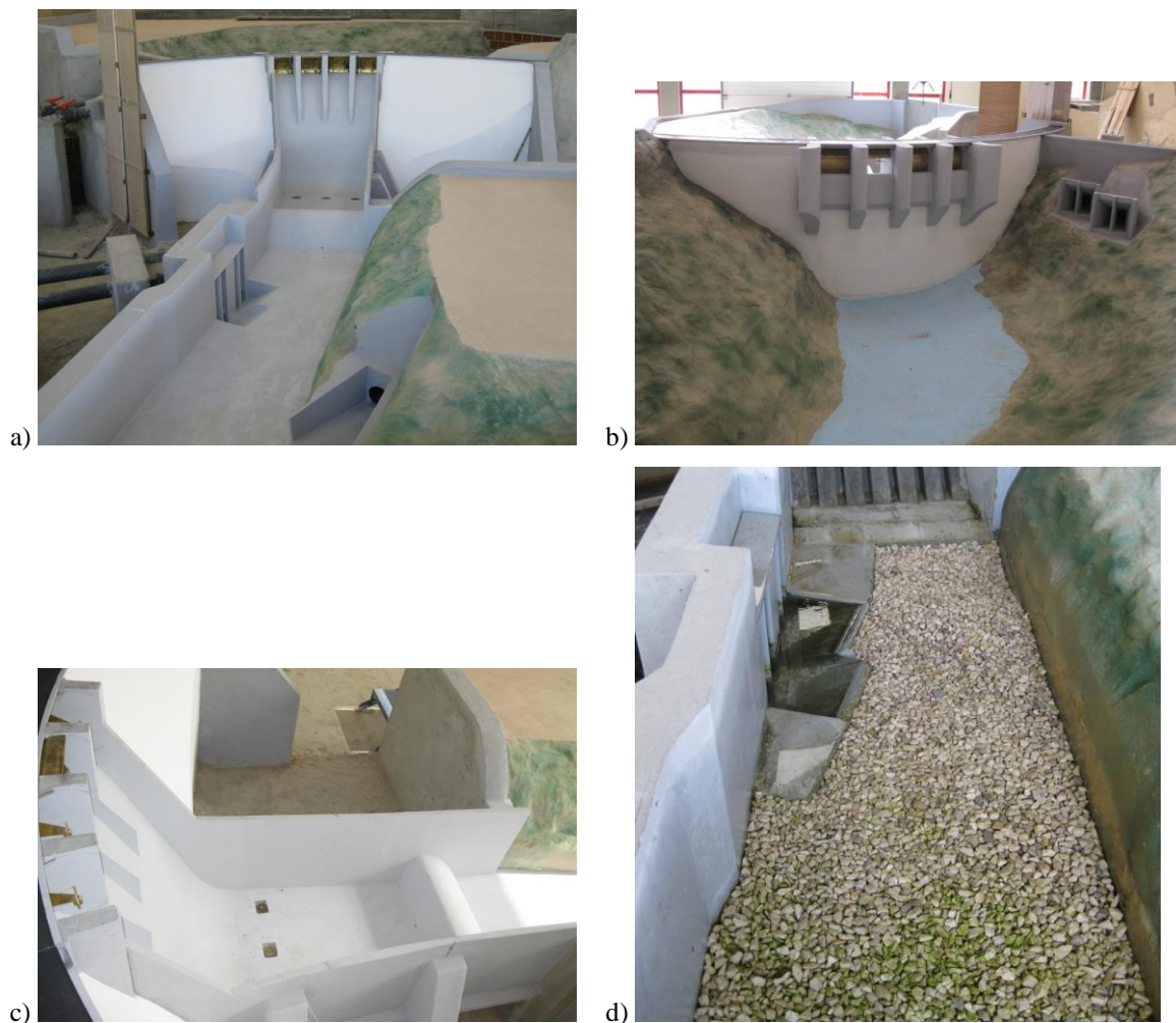
Figure 2: Overview of the Daivões physical model. a) view looking upstream; b) view looking downstream at the reservoir; c) lateral view of the spillway and stilling basin; d) mobile bed used to study erosions
