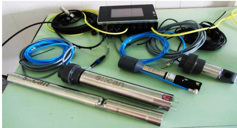
Figure 3.2 – Sensors installed at the Tagus estuary online monitoring station and Con::cube S::CAN controller: spectro::lyser S::CAN (UV-Vis spectrophotometric probe calibrated for COD, TSS and nitrates), ammo::lyser S::CAN (ammonium, nitrates, pH, temperature), condu::lyser S::CAN (conductivity, temperature, salinity) and oxi::lyser S::CAN (dissolved oxygen, temperature).
