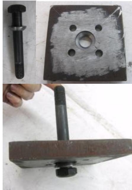
**Figure 3:** Hinged system used in the connection test
