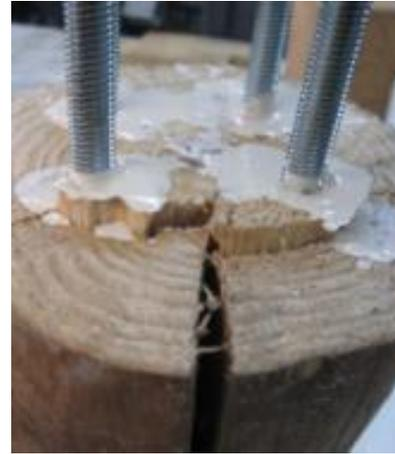
Figure 6: Failure modes observed in the tests
