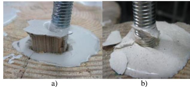
**Figure 1:** Failure of the glued-in rod in the preliminary tests, a) failure on timber, b) failure on glue [14]
