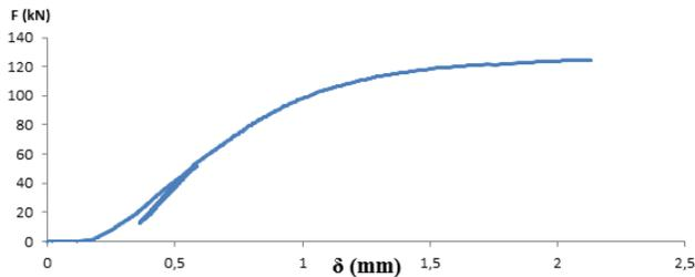
Figure 5: Typical load slip curve of the connection
