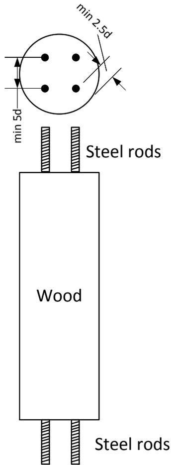
**Figure 2:** Test configuration
