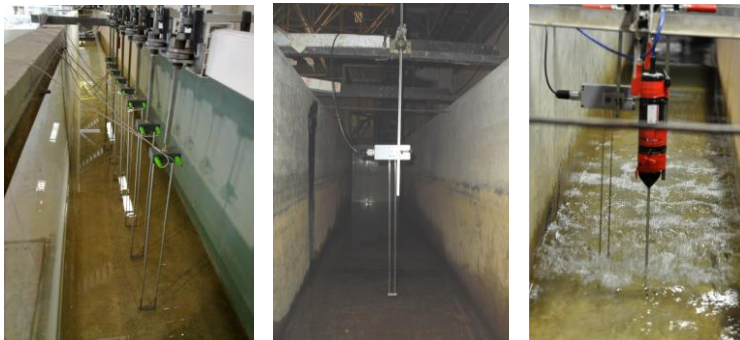
Figure 3. Eight wave gauge mobile structure (left), wave gauge near the wave maker (middle) and ADV probe with wave gauge (right).
