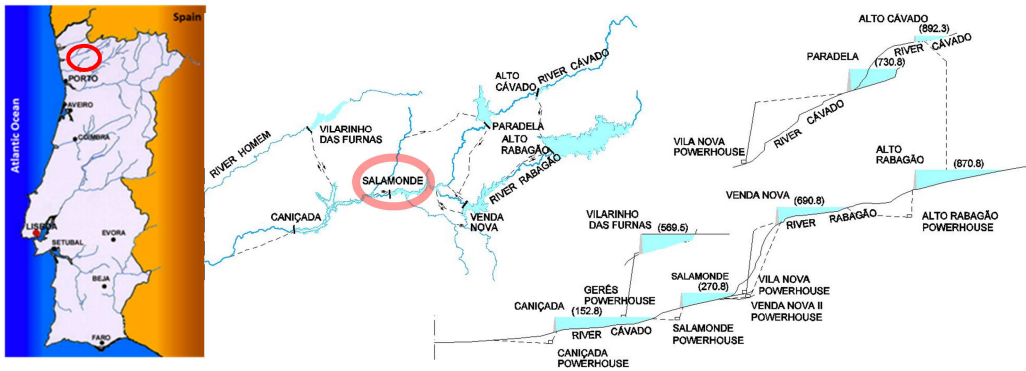
Figure 1. Salamonde II project location and Cávado - Rabagão - Homem Hydroelectric system.
