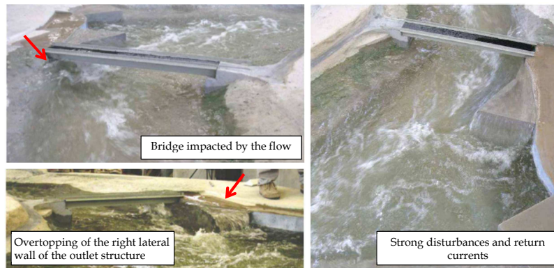
Figure 10. First Alternative Forms . Q_{T=100\text{years}} = 2170 \text{ m}^3/\text{s} ; \text{Level}_{\text{Canica}} = \text{NWL} . Left - Upstream and downstream view. Right - General view of the flow near the outlet structure.
