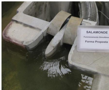
Figure 9. Physical model inlet structure.
