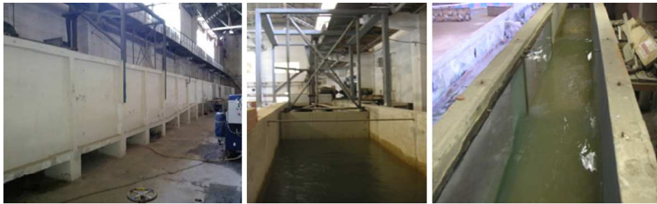
Figure 1. Wave Flume: side view (left), wave maker (middle), view from above (right).
