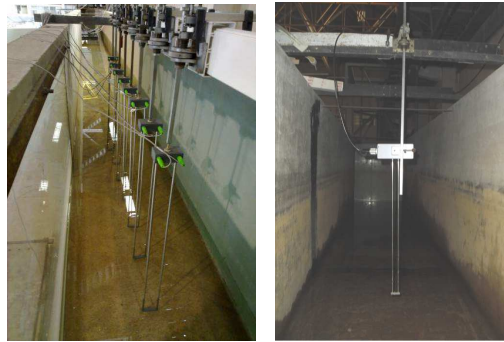
Figure 3. Eight wave gauge mobile structure (left) and wave gauge near the wave maker (right).
