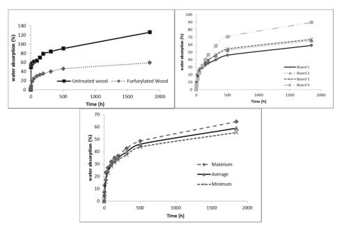
Figure 4: Comparison on water soaking between untreated and treated wood (a) between treated boards (b) along the board 1 (c)
