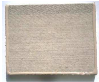
Figure 26 - General appearance of a composite constituted by polyester resin - natural fibre mat on surfaces and unidirectional glass fibres in the core (sample type E)
