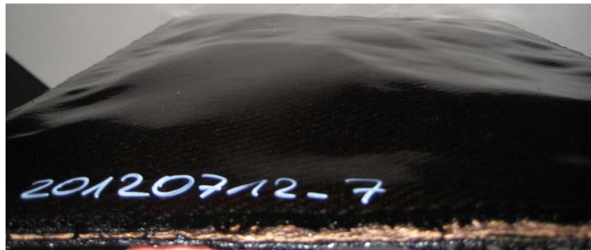
Figure 9 - Baggy cork sandwich panel
