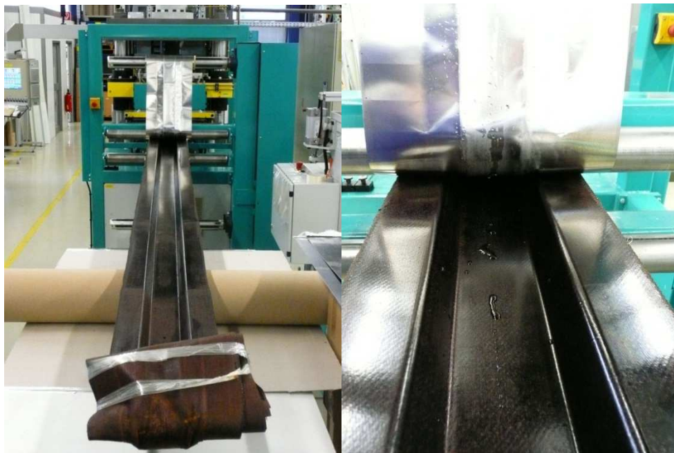
Figure 12 - Production of hat profile in the CCMM
