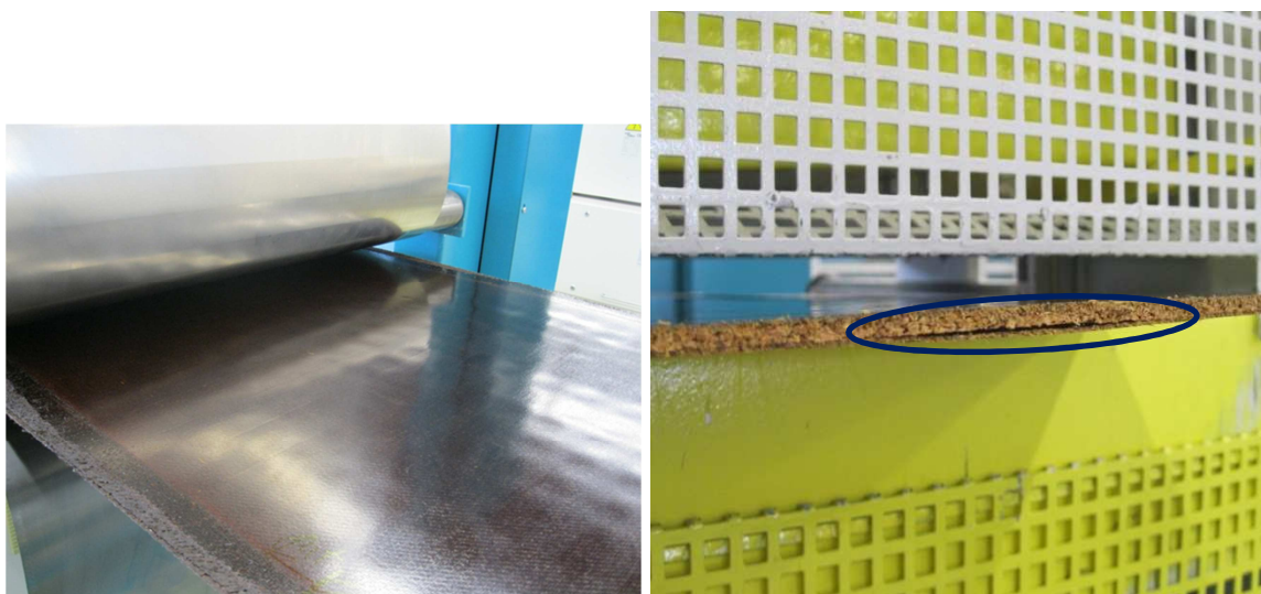
Figure 13 - Bad adhesion between cork and prepregs
