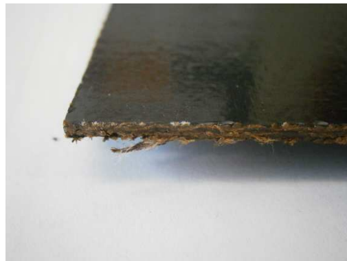
Figure 27 - General appearance a compression-moulded flax+furan (sample type A)
