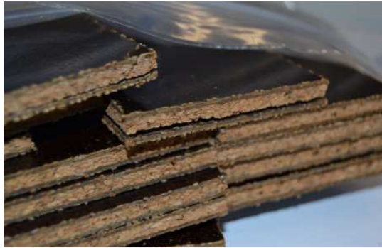
Figure 28 - General lateral appearance of a composite constituted by flax/furan prepreg on surfaces and cork in the core (sample type B)
