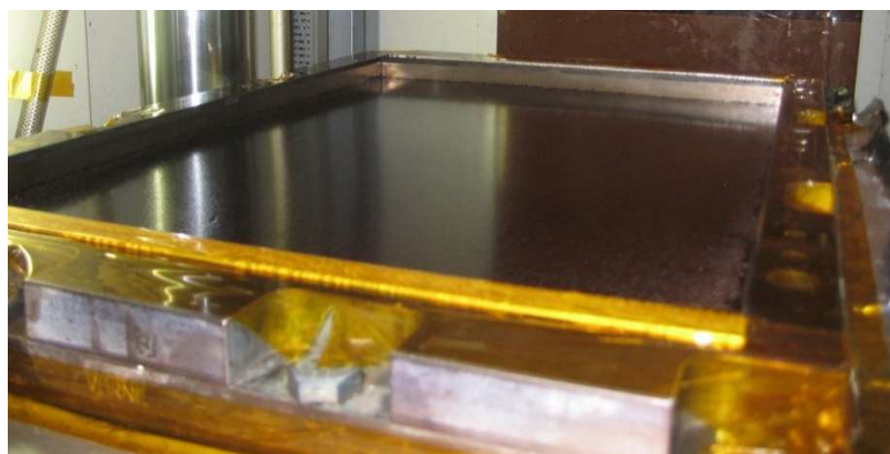
Figure 8 - Processing of natural fibre furan composites with higher fibre weight fraction.
