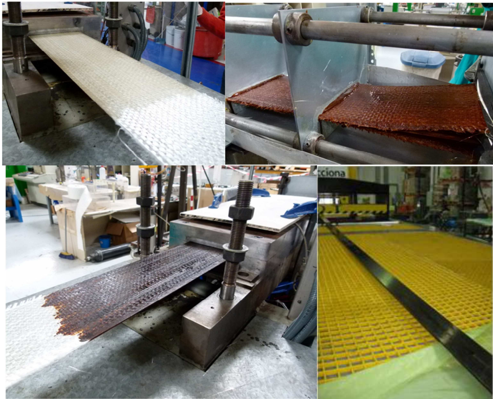
Figure 15 - Pultrusion with furan resin and glass fibre
