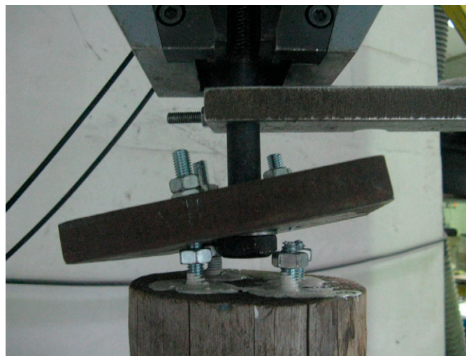
Fig. 5. Failure of a glued-in rod connection
