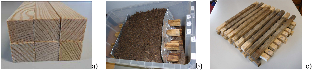
Fig 2 – Preparing wood specimens: a) Selection; b) Process of degradation; c) Look of degraded samples
