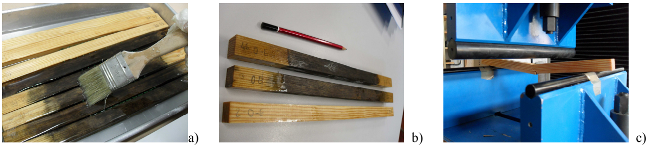
Fig 4 - a) Product application; b) Treated and consolidated specimens; c) Static bending test
