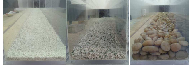
Figure 2. Details of the rough beds used for runs of type R: R1 (left), R2 (center) and R3 (right). View of the channel bed from the downstream section, i.e., right end wall.
