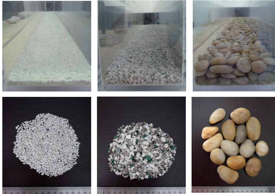
Figure 4. Details of the rough beds used for runs of type R: R1 (left), R2 (centre) and R3 (right). View of the tank bed from the downstream section, i.e. right end wall (top) and sediment samples (bottom)
