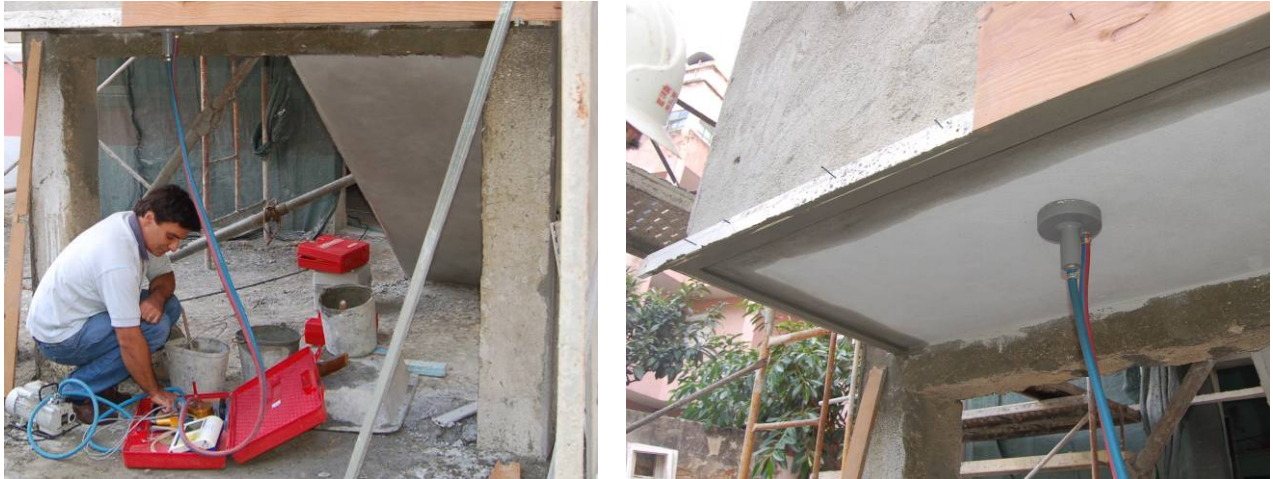
Figure 9: Torrent test in PCM of As
