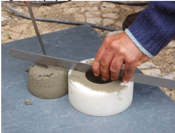
Figure 7: In situ , slump of PCM of AS
