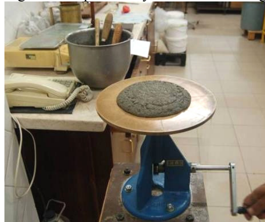
Figure 8: Lab: consistency by flow of PCM
