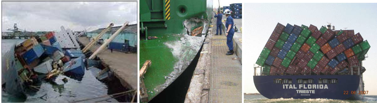
Figure 1. Main hazards of excessive ship movements.
