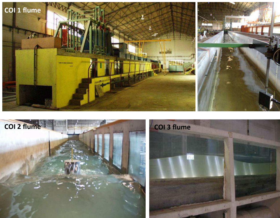
Figure 2 - NPE testing facilities. Irregular wave flumes
