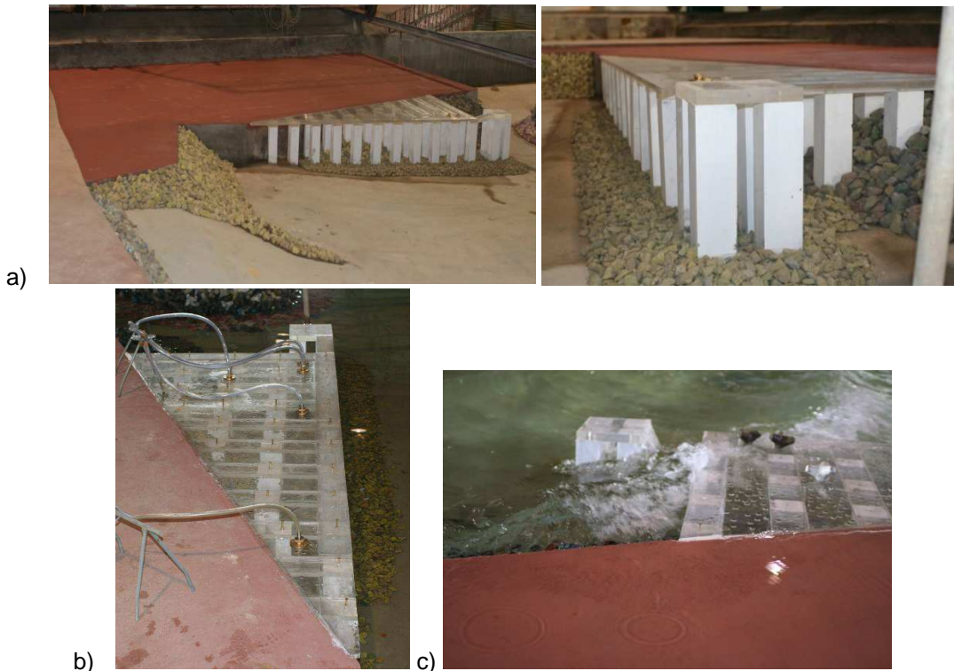
Figure 4 - Ferry boat quay of Vila do Porto Harbour. a) Overview of the designed solution. b) Pressure tests c) Stability and overtopping tests
