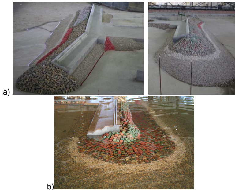
Figure 23 - a) Overview of the design solution b) Detail of a stability and overtopping test
