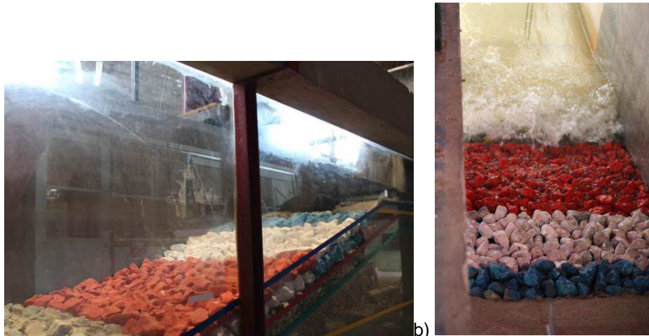
Figure 24 - a) Overview of the 2D model b) View of a test performed with low water level
