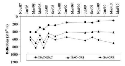
FIG. 14—Mechanical performance of pavement sections with ISAC and natural materials under 47 kN FWD load over time.
