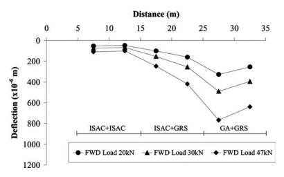
FIG. 13—Mechanical performance of pavement sections with ISAC and natural materials for different FWD loads (date: March 24, 2010).
