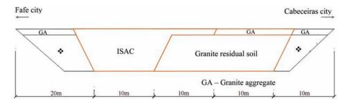
FIG. 10—Longitudinal profile of the full-scale field trial. Gupyt $\Omega$ th by ASTM Int'l (all rights reserved); Thu Sep 27 13:52:55 EDT 2012
