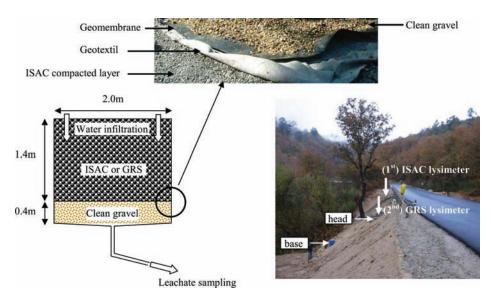
FIG. 12—Lysimeters in the full-scale field trial and schematic representation of these lvsimeters.
