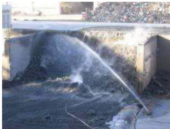
FIG. 2—Cooling of steel slag with water (Roque et al., 2007).
