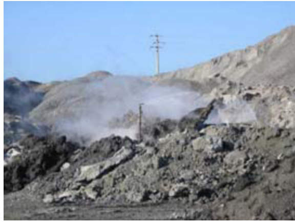
FIG. 3—Cooling of steel slag with air (Roque et al., 2007).
