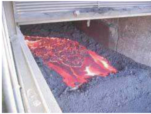
FIG. 1—Emptying of steel slag at the end of the oxidation phase (Roque et al., 2007).
